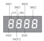
One segment of the display is linked to each input. In the event of failure it switches on according to the following scheme.
